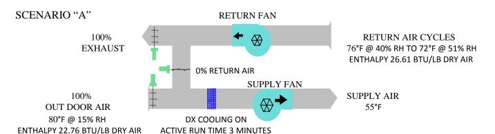
Scenario "A" illustrates a fan system, when the DX cooling compressor is active. Enthalpy comparison determines the heat content of the return air and outdoor air. The system dampers are on full outdoor air, as the total heat content of the outdoor air is approximately 14.5% less than the total heat content of the return air. Selecting the air stream with the lesser heat content causes the refrigeration compressor run time to be minimized.
