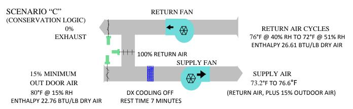
Scenario "C" illustrates the fan system when DX cooling compressor is not active. Cycling the mechanical cooling is based on dry bulb temperature of the space; therefore, the **rest** time of the mechanical cooling will be greater if the supply air is at the lower dry bulb temperature of the return air than the higher outdoor air.
