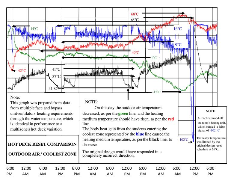
This graph illustrates the heating temperature difference between resetting only from the outside air temperature and resetting from the coolest room of the area served.
