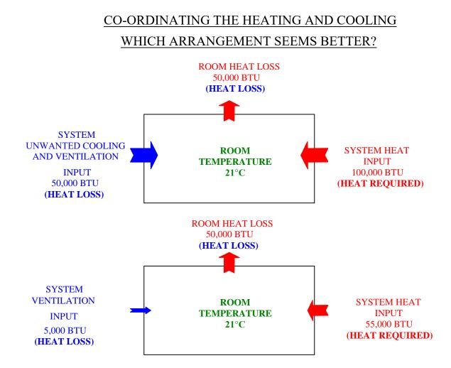
NOTE: When the hot deck, based on only outdoor air reset, is hotter than any zone requires, the cold deck must become colder to compensate for the unwanted heating. When the cold deck is colder than any zone requires, the hot deck must become hotter to compensate for the unwanted cooling.
