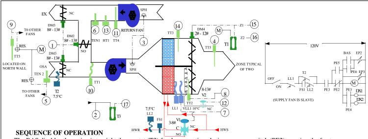
The BAS disables the main air to night thermostat (T3) for day operation closing pressure switch (PE2), causing the fan to run continuously. The BAS holds the dampers in the recirculation position via solenoid valve (EP2) for morning warm-up.
